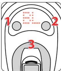
When you touch to "wake up" button if "BL" code is displayed after animated arrows appeared, that means battery of fingerprint reader is weak and need to be replaced with new one.
