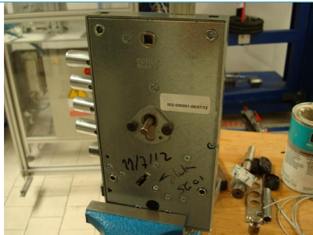
Picture of the lock after the test - load application
