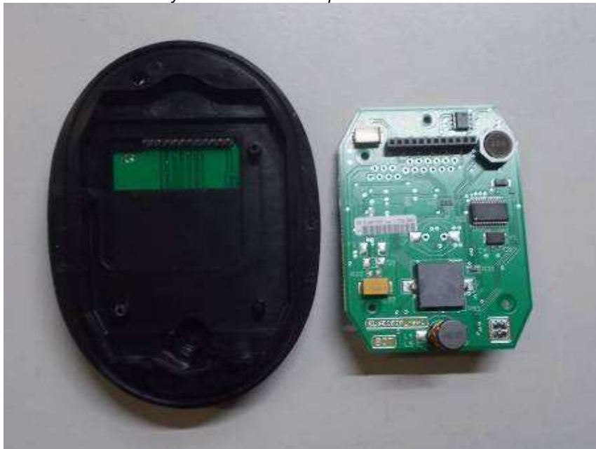
Naked eye visual internal inspection after IPX4 test
