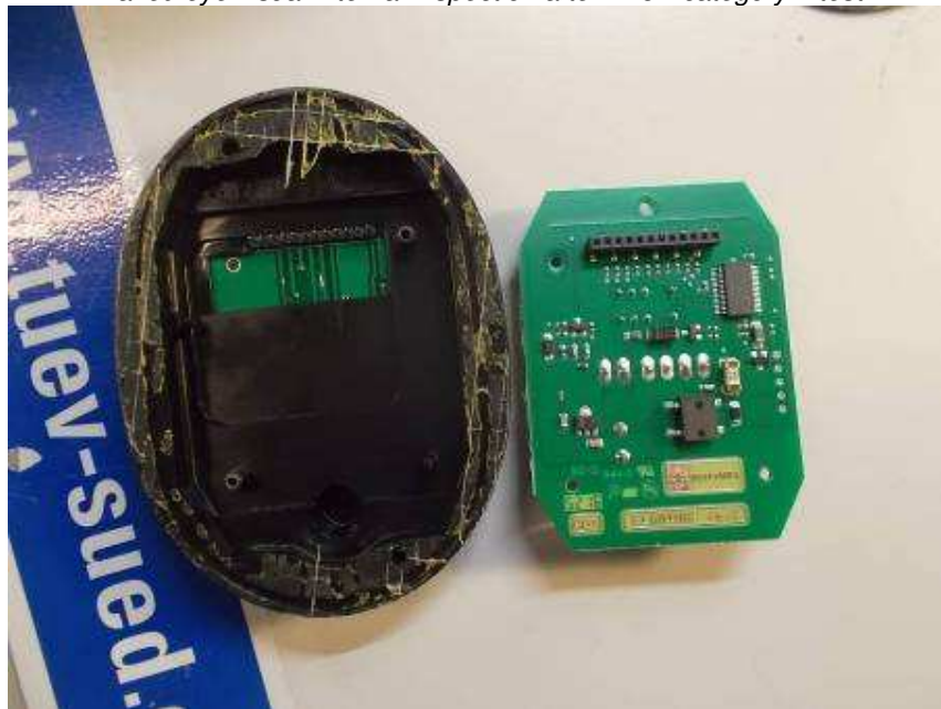
Naked eye visual internal inspection after IP 5X category 2 test
