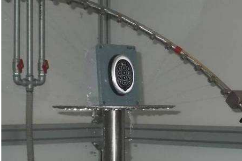
Naked eye visual internal inspection after IPX4 test
