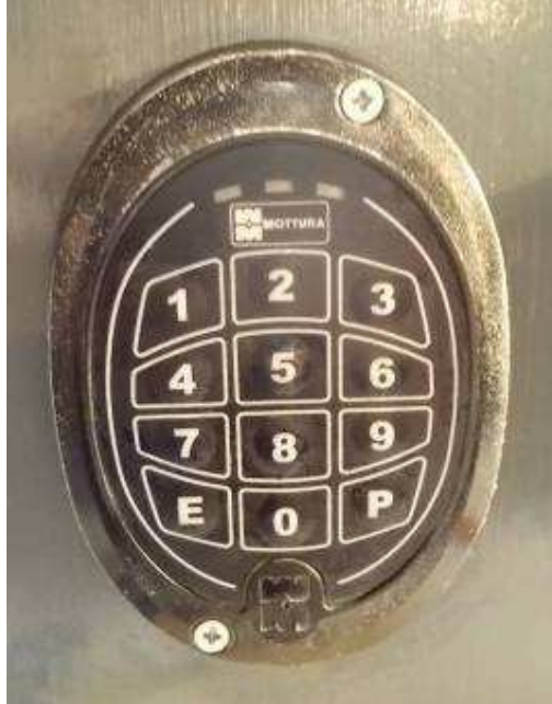
Naked eye visual internal inspection after IP 5X category 2 test
