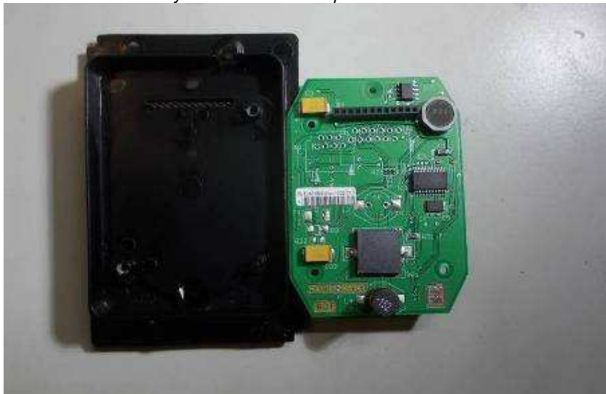
Naked eye visual internal inspection after IPX4 test
