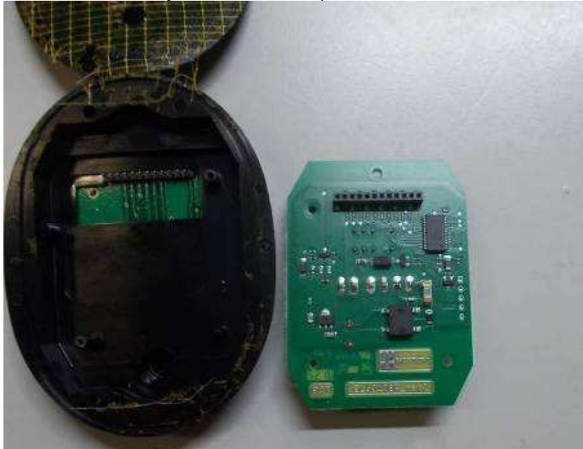
Naked eye visual internal inspection after IPX4 test
