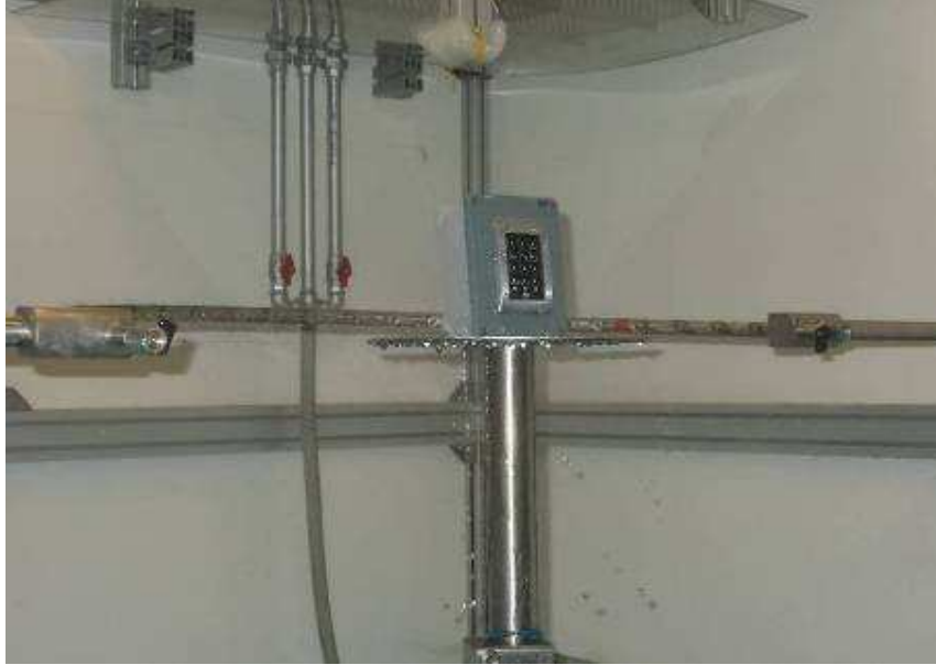
Naked eye visual internal inspection after IPX4 test
